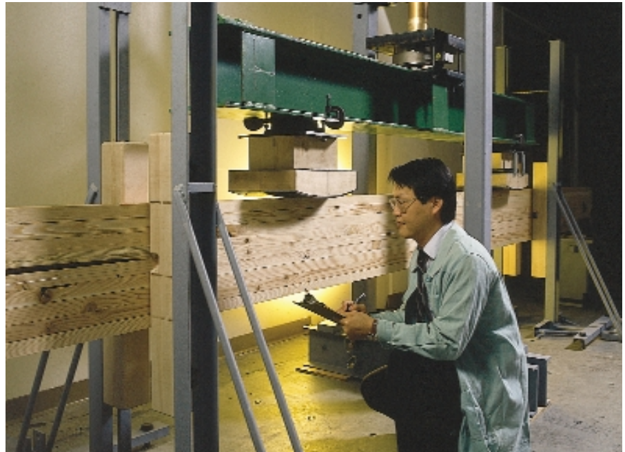
Glulam beam being tested at the APA Research Center.
